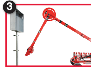
Align with conduit, properly adjust booms
