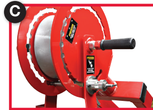
Quick tool-less angle adjustment • Spring loaded pin reduces risk of loss • Faster positioning saves time • Adjusts up to 300°
