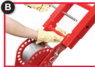
Extended boom • Allows 12' of cable to be pulled from the conduit to the capstan
